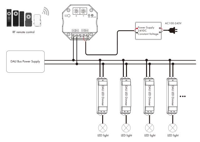
Note: It is recommended to use a 24VDC power supply for the DALI master to reduce the load on the DALI bus power supply.
