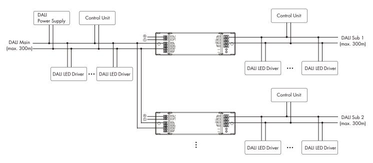
DALI LED driver: include DALI dimming controller, DALI dimming power supply, etc. Control Unit: include DALI master, self-resetting switch, DALI switch panel, DALI sensor, etc.
