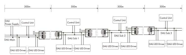
Note: In case of series wiring, up to 3 repeaters can be connected and the DALI bus can be extended up to 1200 meters.
