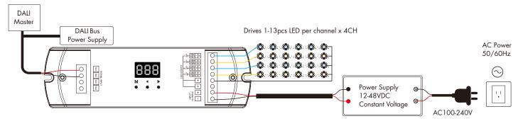
Note: The 3/4 LED channel output is same as 1/2 LED channel.
