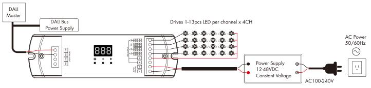
Note: The four output LED channels output is same.
