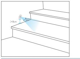
When installing on stairs, install at a height of 8cm or more, as far away from the foot elevation as possible. Make sure that your foot steps up just enough to block the laser and trigger the sensor to light up.
