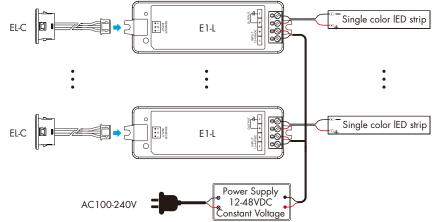
For multiple applications, it is recommended to set the delay time of all laser sensor head to 5 or 10s. Realize the sequential switching control of multiple lights according to the direction of human walking.
