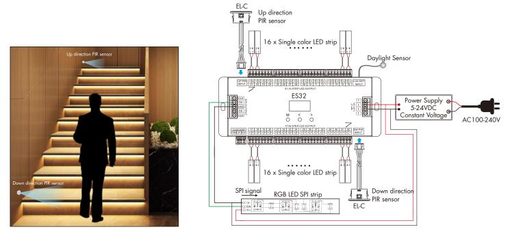
Connect the ES32 sensor stair light controller to two laser sensor head, which are installed at the top and bottom of the stairs. Set the delay time of the laser sensor head to 2s (default).
