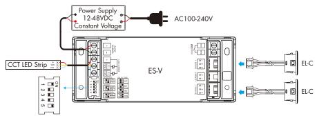
The ES-V constant voltage controller is connected to two laser sensor head which are installed on each side of the corridor. The delay time of the laser sensor head is set to 2s (default value), Set DIP switch 3 to OR (light on when any one of the sensing inputs is on). Set DIP switch 4-5 to 30, 60 or 180s.
