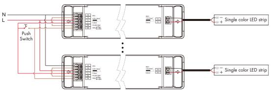
The provided AC Push-Dim interface allows for a simple dimming method using commercially available non-latching(momentary) wall switchs.
