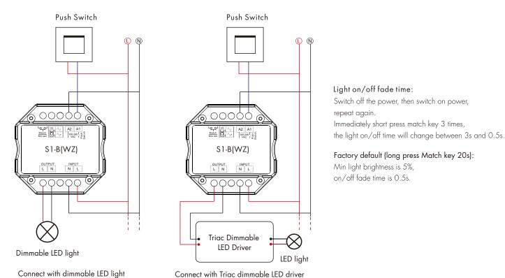
Note: When calculating the maximum number of load lamps or drivers, the input power or input current parameters of a single lamp or driver must be used, the output power parameters can not be used.
