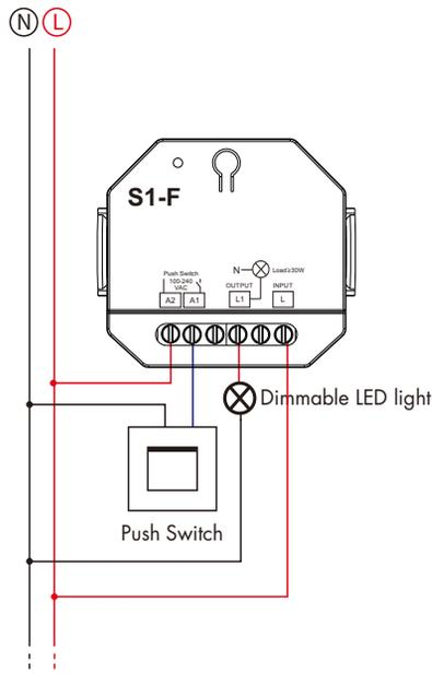
**⚠ Caution:** Please carefully ensure all wire connections and polarities are correct and secure before applying power, otherwise this dimmer will be damaged.
