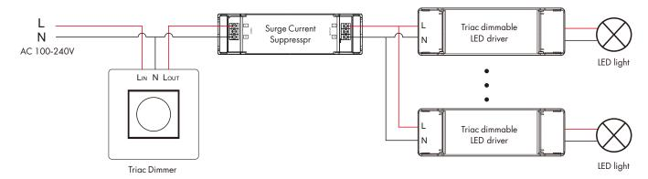
Note: It is recommended that the total power of the connected LED dimmable drivers or LED dimmable luminaires load does not exceed 1920W and the total working current does not exceed 8A.
