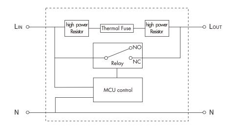
The moment the product is powered up, two 7.5 $\Omega$  high power resistors are connected in series between LIN and LOUT to reduce the load power-on surge current. After about 40ms, the relay switch will be engaged and the LIN and LOUT will go through.
