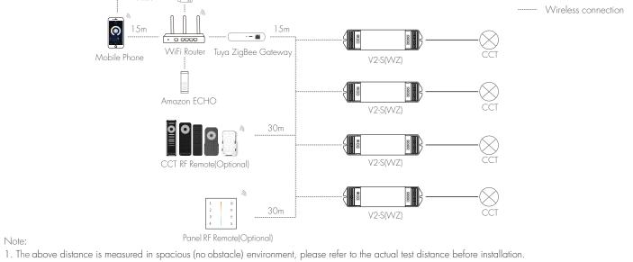
2. Users must use the Tuya ZigBee gateway to realize remote control and voice control.
