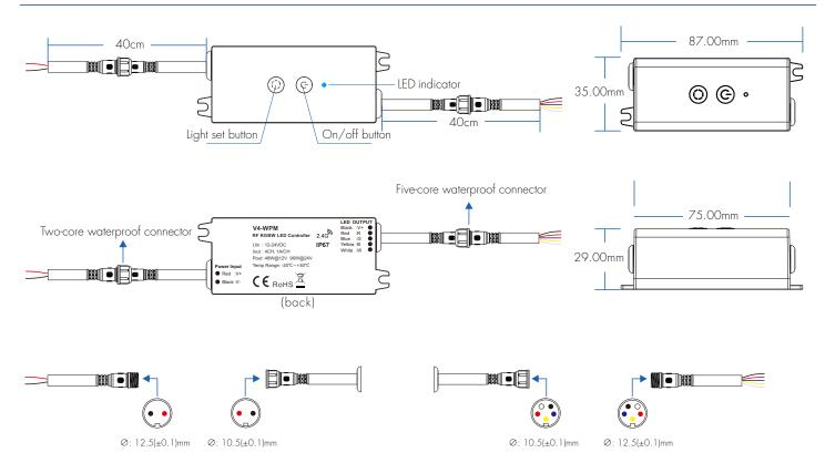
NOTE: When installing, align the insert and tighten the nut.
